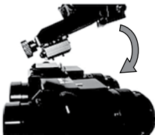
FIGURE 2-4. ATTACHING THE BINOCULAR TO THE MOUNT
